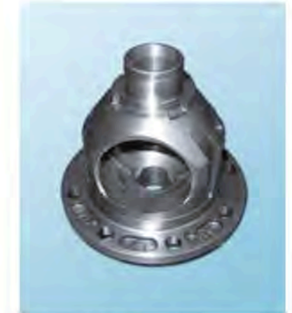
Differential housing Complete all the processing of the difference shell in order, Ensure that the position of the flange surface and the journal at both ends is 0.02mm, Journal diameter tolerance 0.03mm, CPK ≤ 1.33
