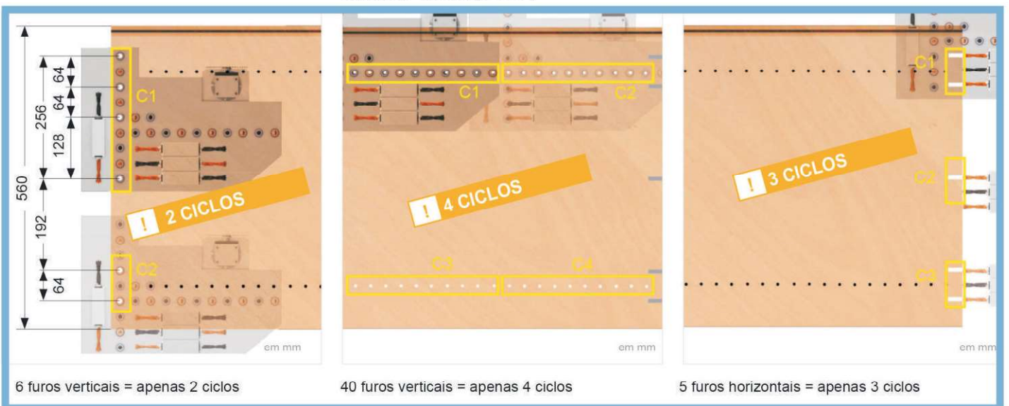
High-Speed 1500 a 7500 rpm V21 – 21 mandrils verticais, 8 mandrils horizontais, 1 senha de ranhura \varnothing 125 mm ( 0^\circ / 90^\circ )
