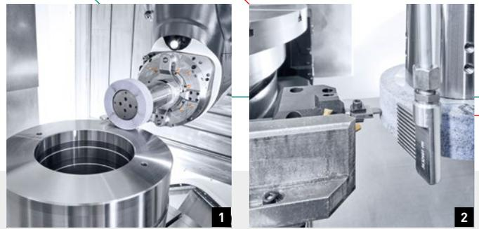
1: Detecting of components via spindle load
