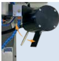
Programmable coolant nozzle
